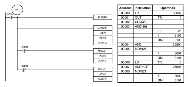
Although two ADD(30) can be used together to perform eight-digit BCD addition, ADDL(54) is designed specifically for this purpose.
